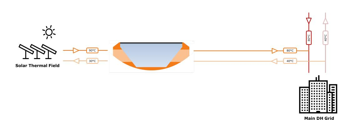
Possible Integration of a PTES in a DH Grid with low temperatures
