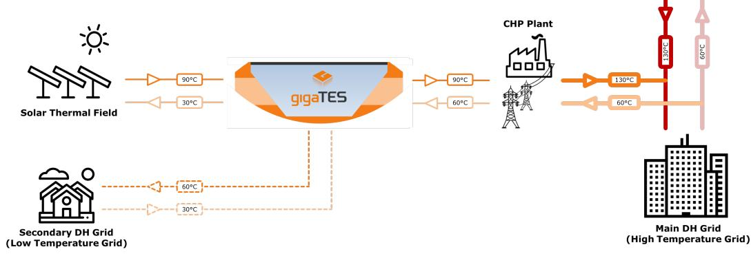
Possible Integration of a giga\_TES in a DH grid with high temperatures
