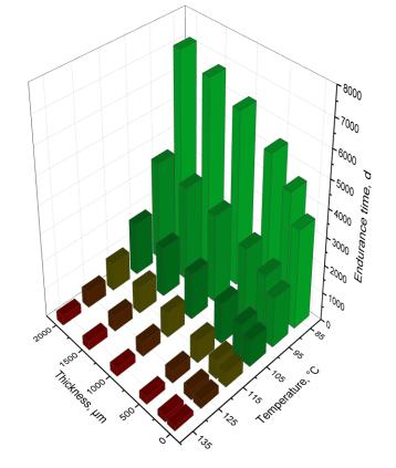
Grabmann, M.K., Wallner, G.M., Grabmayer, K., Buchberger, W., Nitsche, D. (2018). Effect of thickness and temperature on the global aging behavior of polypropylene random copolymers for seasonal thermal energy storages, Solar Energy, 172, 152-157. (doi: 10.1016/j.solener.2018.05.080)
