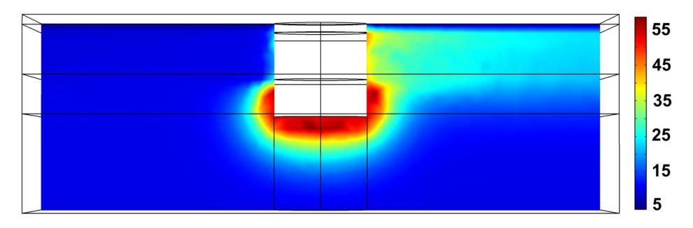
Example: temperature distribution due to flowing groundwater (COMSOL)
